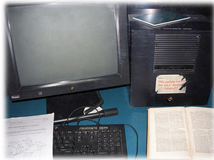
*Figure 1. This NeXT Computer was used by Berners-Lee at CERN and became the world's first Web server. (Coolcaesar)*
